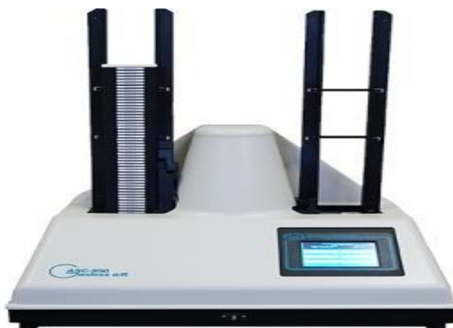
Figure 2.4. The \alpha/\beta counter employed for the assessments of several environmental sample
